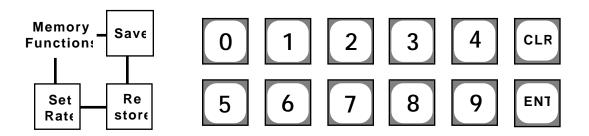
A Save to register 62, for example, is obtained by pressing Save, 6, 2, ENT. During this operation a message will appear on the LCD display. This Save operation will copy the current TBC control values and the current transition rate into register 62. Save operations have no effect on the values being sent to the TBC and hence no effect on the on screen video.
