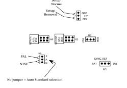
**SMPTE** Input For example, if you are feeding a BetaCam VTR, Y, R-Y, B-Y, (YUV).
