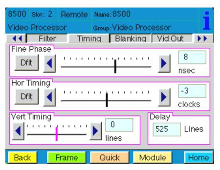
The **Blanking** menu shown below allows you to adjust the output blanking of the module with the following controls:
