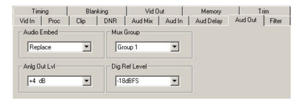
**8415**: Use the **Aud Out** menu shown below to adjust the following audio output parameters:
