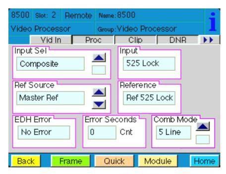
The **Proc** menu shown below allows you to adjust the following video processing parameters for the signal:
