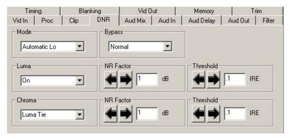
**Adaptive** – this mode requires manual settings of all parameters. Fine detail is preserved and motion is removed. Best used for signals with less motion and results viewed with the Show Noise function and a waveform monitor. The Adaptive controls are shown in the figure below.
