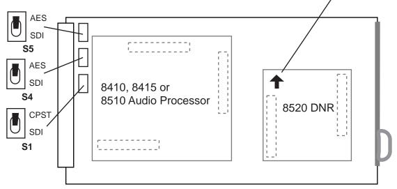
Submodule Installation and BNC Configuration Switches
