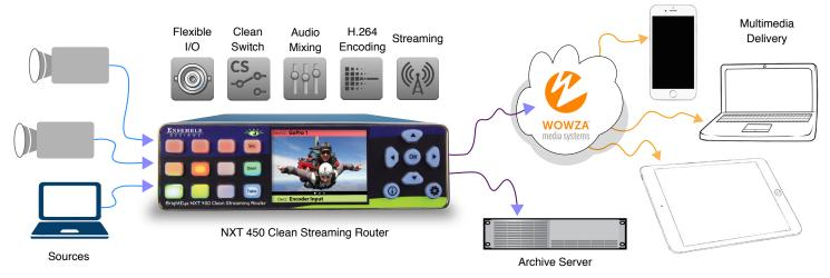
Connect your sources, the NXT 450 will switch between inputs, automatically convert formats, Encode and Stream. It's easy to configure and control through the web interface.
