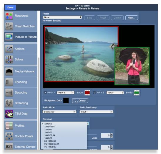
Note: PiP-Efx allows signals of different formats and frame rates to be combined together simply by setting the PiP-Efx output standard. The input signals (PiP In A and PiP In B) can be any combination of formats. They will be automatically converted to your chosen output standard, regardless of their incoming formats.
