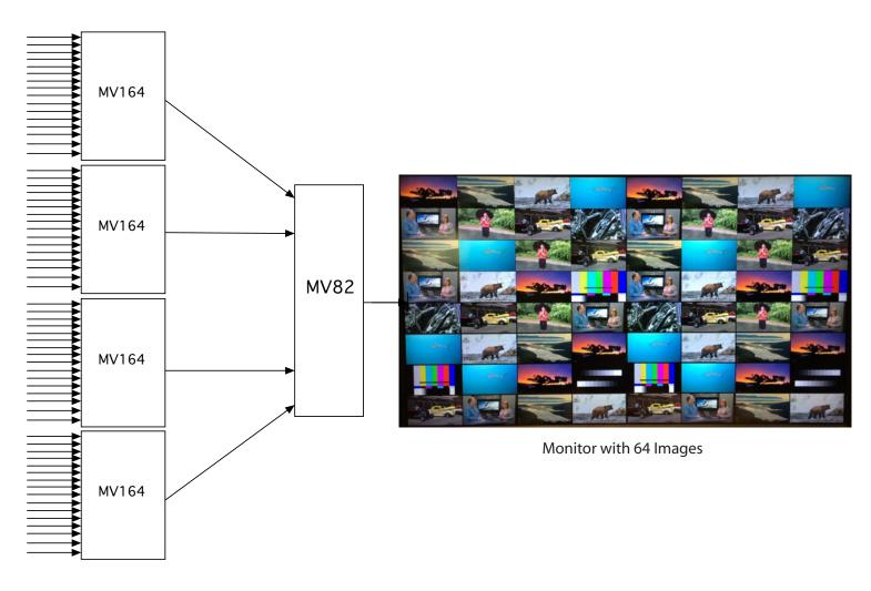
This unique architecture not only allows 32 or 64 sources to be displayed on a single screen, but operationally, allows either 8 or 16 of those sources to be brought forward from the overall display, and then any one cell within those 8 or 16 sources to brought to full screen for detail analysis and/or isolated audio from that cell. This can be accomplished via the web browser interface or GPI trigger.
