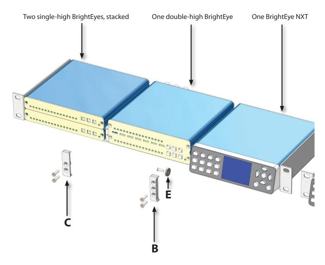
Illustration of BrightEyes and a BrightEye NXT installed in the rack mount, using a BrightEye to BrightEye front retainer (**C**), a BrightEye to NXT front retainer (**B**) and an NXT Retainer Washer (**E**), exploded view
