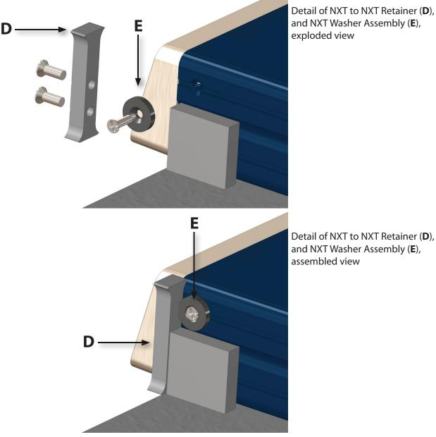
Detail of NXT to NXT Retainer (D), and NXT Washer Assembly (E), exploded view
