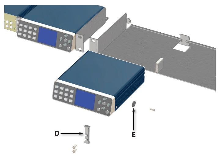
Illustration for installing a BrightEye NXT, using a NXT to NXT front retainer (**D**), and a NXT Retainer Washer (**E**), exploded view
