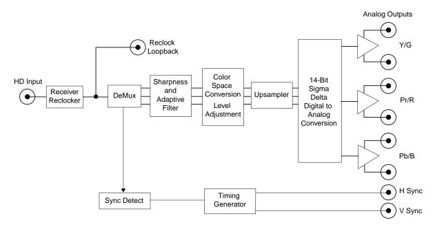
7200 HD Digital to Analog Converter Functional Block Diagram
