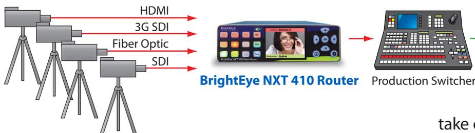
Add more inputs to your production switcher or master control switcher. Feed cameras and other SDI and HDMI sources to a BrightEye NXT 410 Router and take one or more of the router outputs into the production switcher or master control switcher. This is also a great way to integrate HDMI signals into an SDI workflow.
