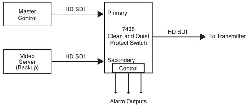
*Redundant Auto-Switched Conversion with 7435 Module*
