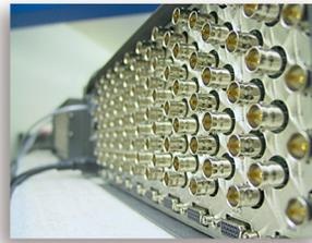
Avenue frames handle 270 Mb/s, 1.5 Gb/s and 3 Gb/s signals, audio and MPEG signals. Used worldwide in broadcast, mobile, production, and post.
