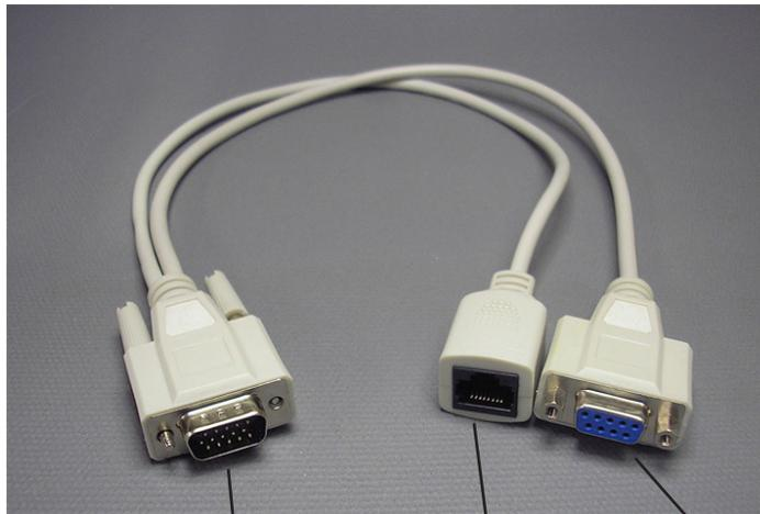
Connect the male 15 pin D connector to the female 15 pin D connector on the rear of the Avenue frame that corresponds to the 9455/7435 clean switch module.
