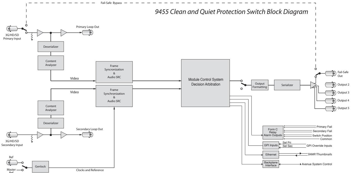
The block diagram, above and on the following page, illustrates the signal flow of the 9455. Note that in the event of power failure, the passive relay passes the primary input to the Relay Protected Output.
