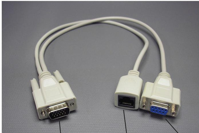
Connect the male 15 pin D connector to the female 15 pin D connector on the back of the frame that corresponds to the clean switch module
