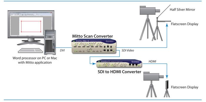
The BrightEye Mitto scan converter can be used with applications such as Microsoft Word or PowerPoint<sup>™</sup> to provide an effective teleprompting solution without breaking the bank.
