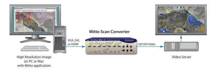
Use BrightEye Mitto to output detailed maps to 3 Gb/s HD video. Connect your Mac or PC to the BrightEye Mitto through the VGA, DVI or HDMI port on your computer. Mitto outputs full 1080p HD video at 3 Gb/s for maximum detail.
