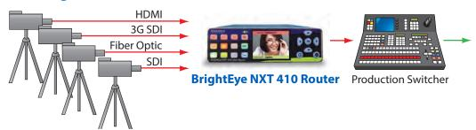
Add more inputs to your production switcher or master control switcher. Feed cameras and other SDI and HDMI sources to a BrightEye NXT 410 Router and take one or more of the router outputs into the production switcher or master control switcher. This is also a great way to integrate HDMI signals into an SDI workflow.
