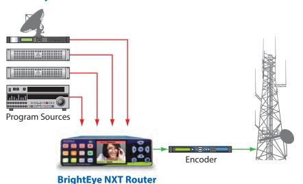
Use the BrightEye NXT Router as a cuts-only master control, on the ground or in the air. Great for helicopters, sports and ENG, the BrightEye NXT Router has built-in frame syncs that let you use sources that don't have a reference. The router's output is clean and guiet, switching seamlessly between sources. Downstream devices such as routers and encoders receive a consistent video
