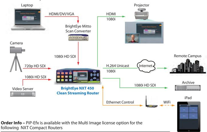
**BrightEye NXT 450** Compact Router with H.264 Encoder/Decoder and U/D/C
