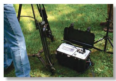
When equipped with Bidirectional fiber, BrightPak supports outbound sound and picture, with return video, sound, and ifb
