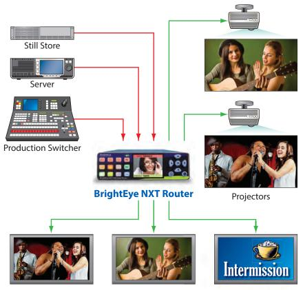
Use the BrightEye NXT Router for live events and sports to route signals to monitors, switchers and projectors. The router's outputs can be easily configured to be in time with house, even when there are asynchronous sources on the input. Switch seamlessly between fiber optic, HDMI and SDI signals.
