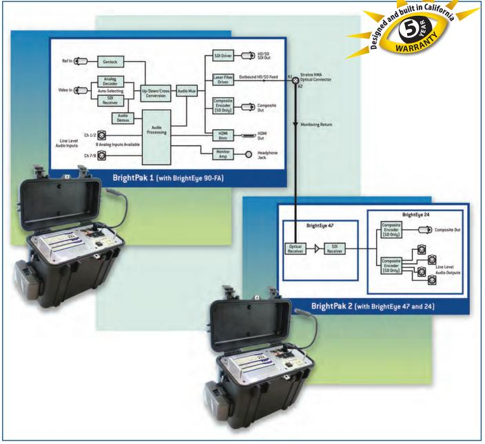
In this example two BrightPaks are used for outdoor field news acquisition. One BrightPak is populated with a BrightEye 90-FA Up/Down/Cross Converter and is processing an HD or SD camera feed. The BrightEye 90-FA upconverts or cross converts the signal as needed to the desired HD format. For example, if the desired output is 720p, any input delivered to the BrightEye 90-FA (SD or HD) would be converted to 720p. Audio levels and video levels can be adjusted.
