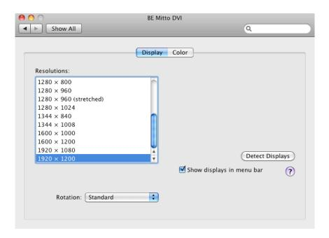
3. From the Resolutions control, set the resolution to be sent to the Mitto. For the best video output from BrightEye Mitto, select  $1920 \times 1200$  or  $1024 \times 768$ .  $1920 \times 1200$  is the maximum resolution that Mitto accepts.
