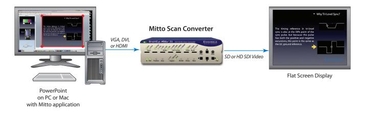
The above illustrates how you can connect your Mac or PC to the BrightEye Mitto through the VGA, DVI or HDMI port on your computer. Mitto outputs composite, SD or HD video that can be fed into a monitor or production switcher.
