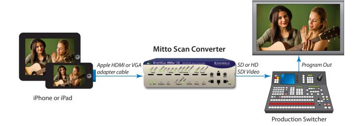
The above illustrates how you can connect your iPhone  $^{\text{m}}$  or iPad $^{\text{o}}$  to the BrightEye Mitto and output HD or SD SDI video for use in production or post.
