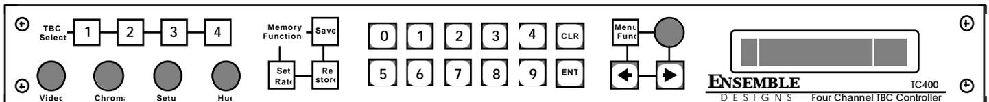
The TC400D is a 1 RU chassis with a depth of 12 inches. Removable ears are included for installation in a conventional 19" equipment rack. The ears can also be mounted with a 3/4" set-back which allows them to serve as mounting brackets when the TC400D is installed from behind in a wooden console. The TC400D is powered by a small, modular transformer.
