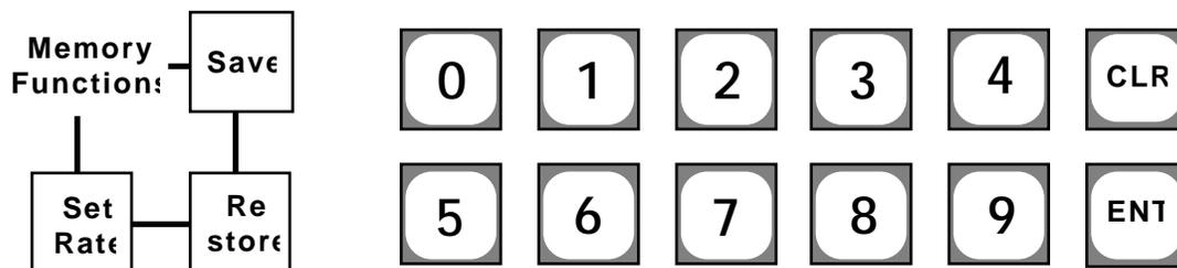
A Save to register 62, for example, is obtained by pressing Save, 6, 2, ENT. During this operation a message will appear on the LCD display. This Save operation will copy the current TBC control values and the current transition rate into register 62. Save operations have no effect on the values being sent to the TBC and hence no effect on the on screen video.
