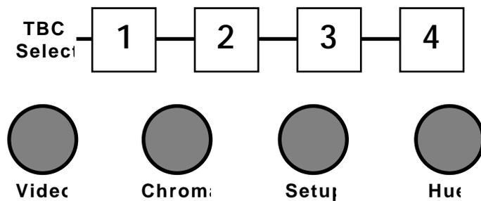
For each of the four controllable values there is a nominal, or detent value which can be programmed through a menu function. This value is in the middle of the range of each control. Pressing and holding a TBC Select button for at least one second will reset all four of the control values for that machine to those nominal values.
