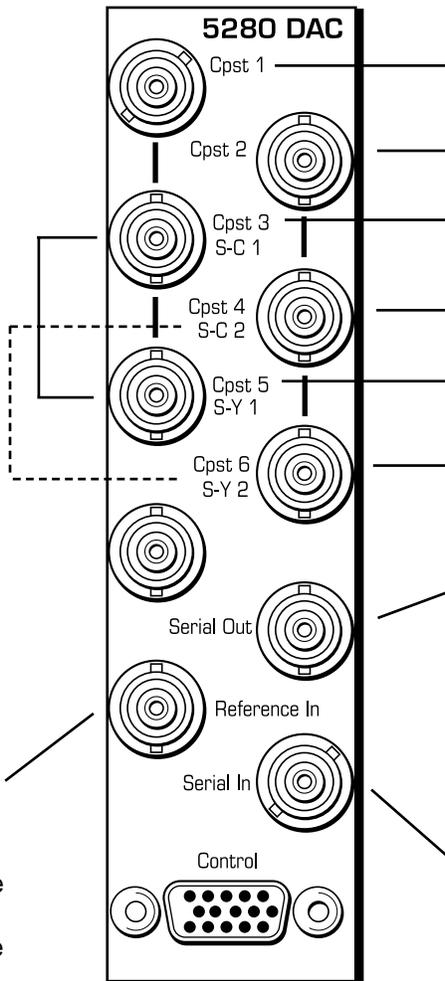
For **Composite** output operation: Connect the six output BNCs to analog composite destinations.
