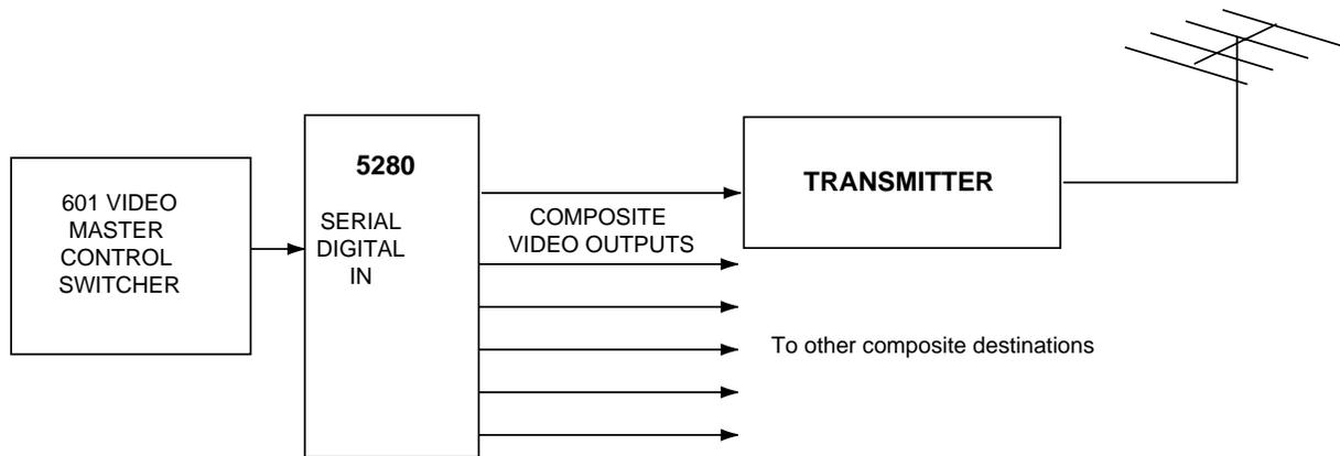
Serial Digital to Composite Encoder for Transmission Application
