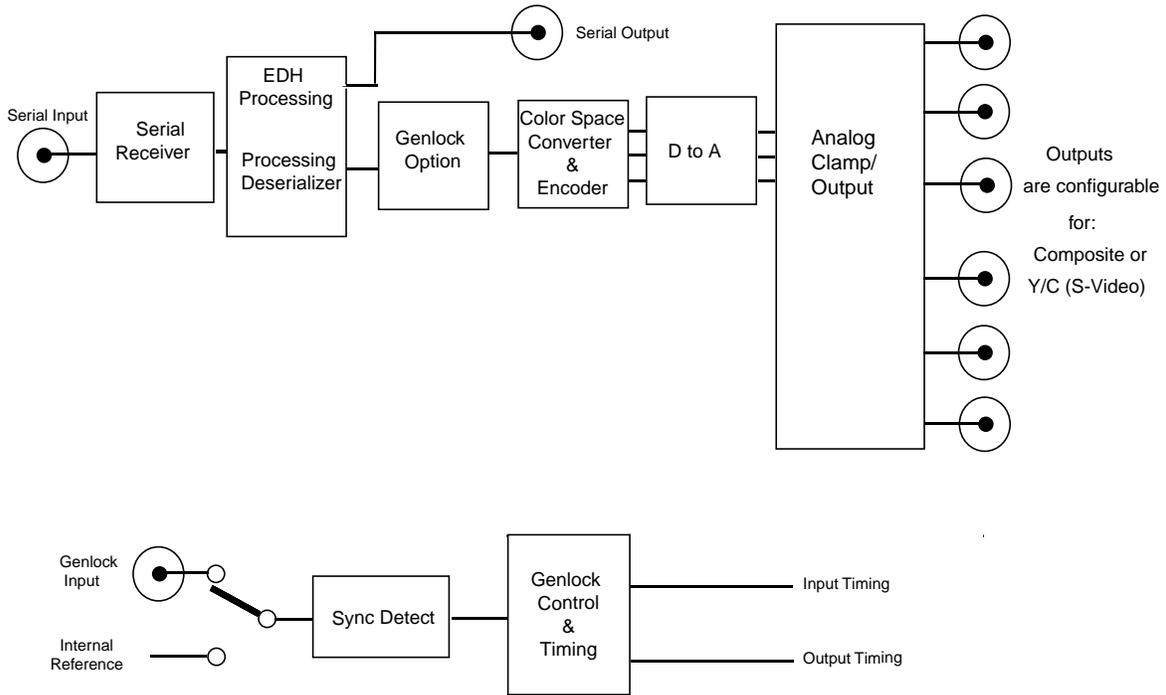
**5280/5210 Digital to Analog Composite Video Converter Functional Block Diagram**
