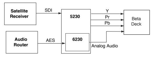
Satellite Receiver and Audio Router Feeding a Beta Deck
