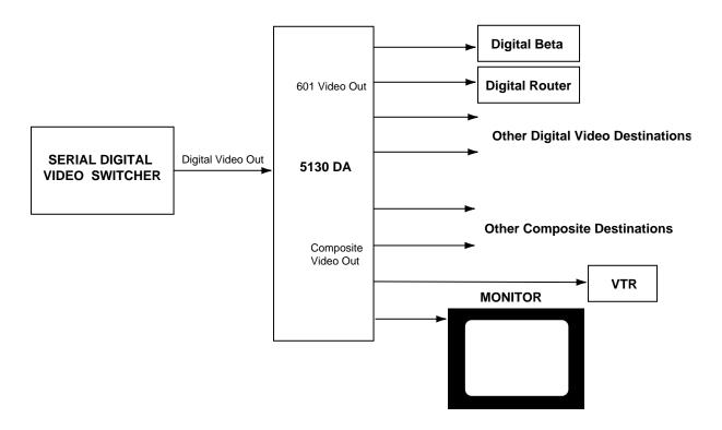
5130 Serial DA with Monitor Outputs Application
