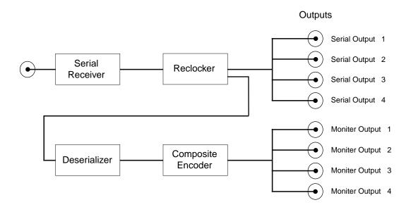
5130 Reclocking DA with Monitor Outputs Block Diagram
