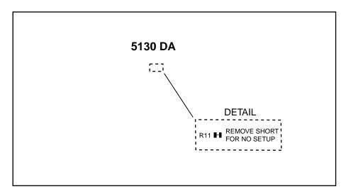
Remove Short on R11 for No Setup in 525 Mode
