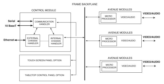
Figure 1. The control modules interface to the frame backplane for controlling the Ethernet TCP/IP connection, the AveNet LAN connection, the AveNet Over IP function and the serial communications port.
