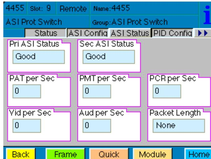
The **PID Config** menu is used for configuring the PID-specific targeting ability of the 4455. If you have chosen **PID Specific** from the **Config** menu's **ASI Test** pull-down menu, you are in PID Specific Mode. When in this mode, you can assign and configure up to 32 "PID Watchers" or "Targets," each tasked to monitor the data rate of their specific PID Target in an ASI signal. These are running in parallel, so there is no need to configure all 32 targets.
