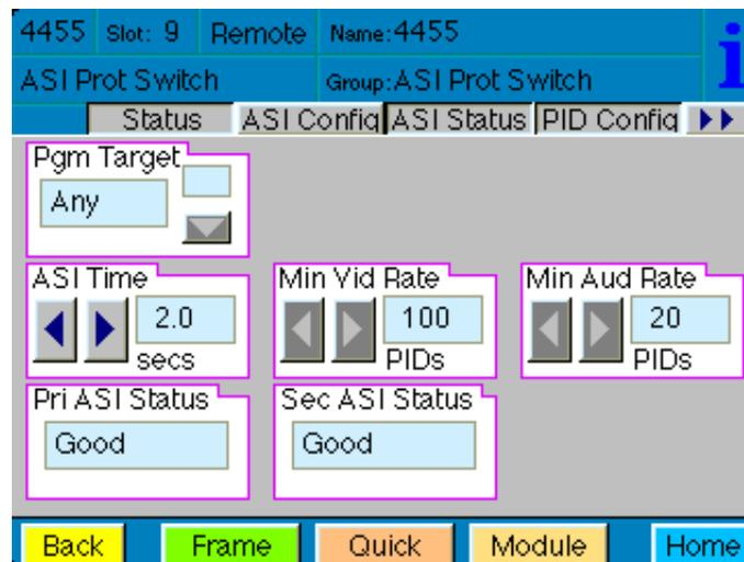
The **ASI Status** menu shown below displays a breakdown of critical elements of analysis with a display of live results. The displayed values for the rate (in PIDs per second) for the video and audio can be used as a guide to setting the **Min Vid Rate** and **Min Aud Rate** values in the **ASI Config** menu for a particular system or installation. Additionally, the **ASI Status** menu shows the status of the following parameters:
