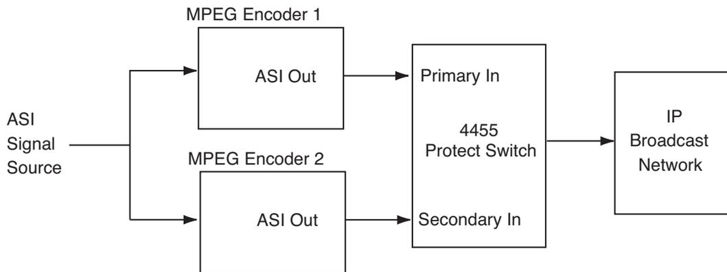
**Redundant Auto-Switched Conversion With 4455 Module**
