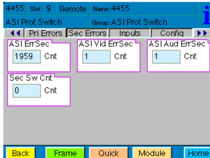
The **Sec Errors** menu shown below displays the amount of time in seconds that each of the enabled error conditions have been present after detection on the Secondary as well as the number of times the switch has switched from the Primary feed to the Secondary feed (**Sec Sw Cnt**).
