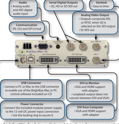
The BrightEye Mitto Family has multiple models to choose from so you can select the perfect combination of features and price for your video facility. The diagram above shows Mitto model BEM-1. Rear connections vary with other models.
