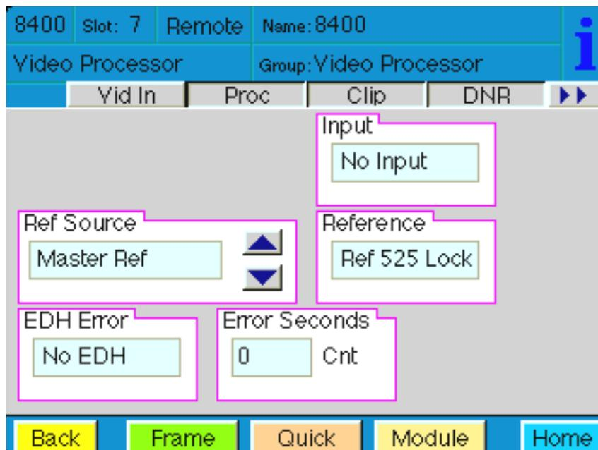
The **Proc** menu shown below allows you to adjust the following video processing parameters for the signal. For numerical choices, use the slider control to select a value or enter a value into the number field at right and press the **Enter** key on your PC.
