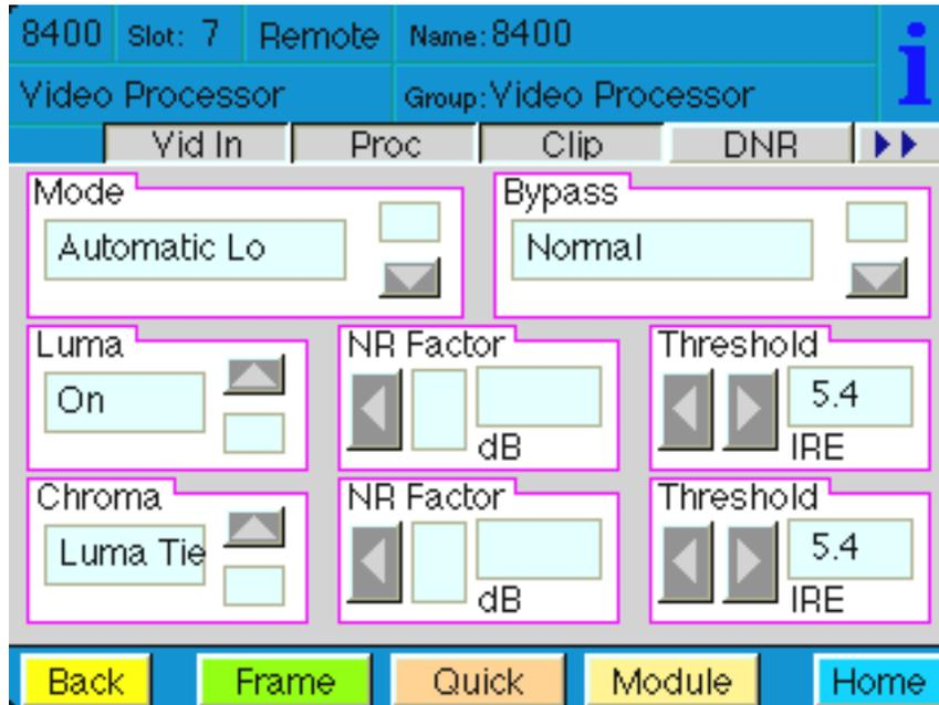
**Adaptive** – this mode requires manual settings of all parameters. Fine detail is preserved and motion is removed. Best used for signals with less motion and results viewed with the Show Noise function and a waveform monitor. The Adaptive controls are shown in the figure below.
