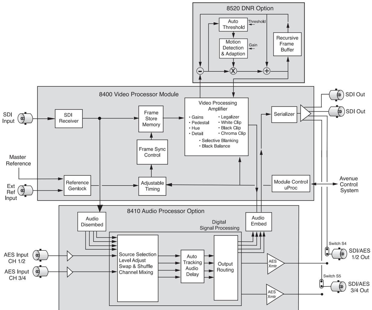
Alternately, the 8415 or 8510 Audio Processor Options can be used with the 8400.
