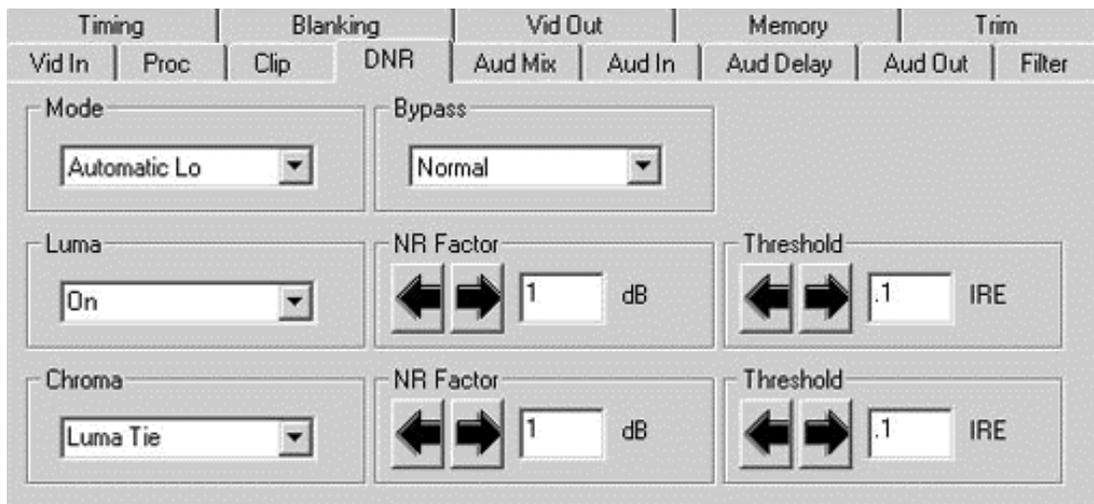
**Adaptive** – this mode requires manual settings of all parameters. Fine detail is preserved and motion is removed. Best used for signals with less motion and results viewed with the Show Noise function and a waveform monitor. The Adaptive controls are shown in the figure below.
