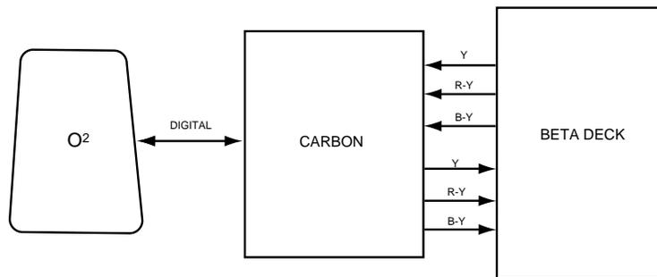
If the Carbon Input option is not installed, an alternate method of capturing video into the O<sup>2</sup> is available. This method allows you to route the Carbon key input directly into the O<sup>2</sup>'s analog composite input by connecting your analog video source into the Carbon Key In BNC and selecting O<sup>2</sup> Cmpst Src (O<sup>2</sup> Composite Source) in the menu selection.
