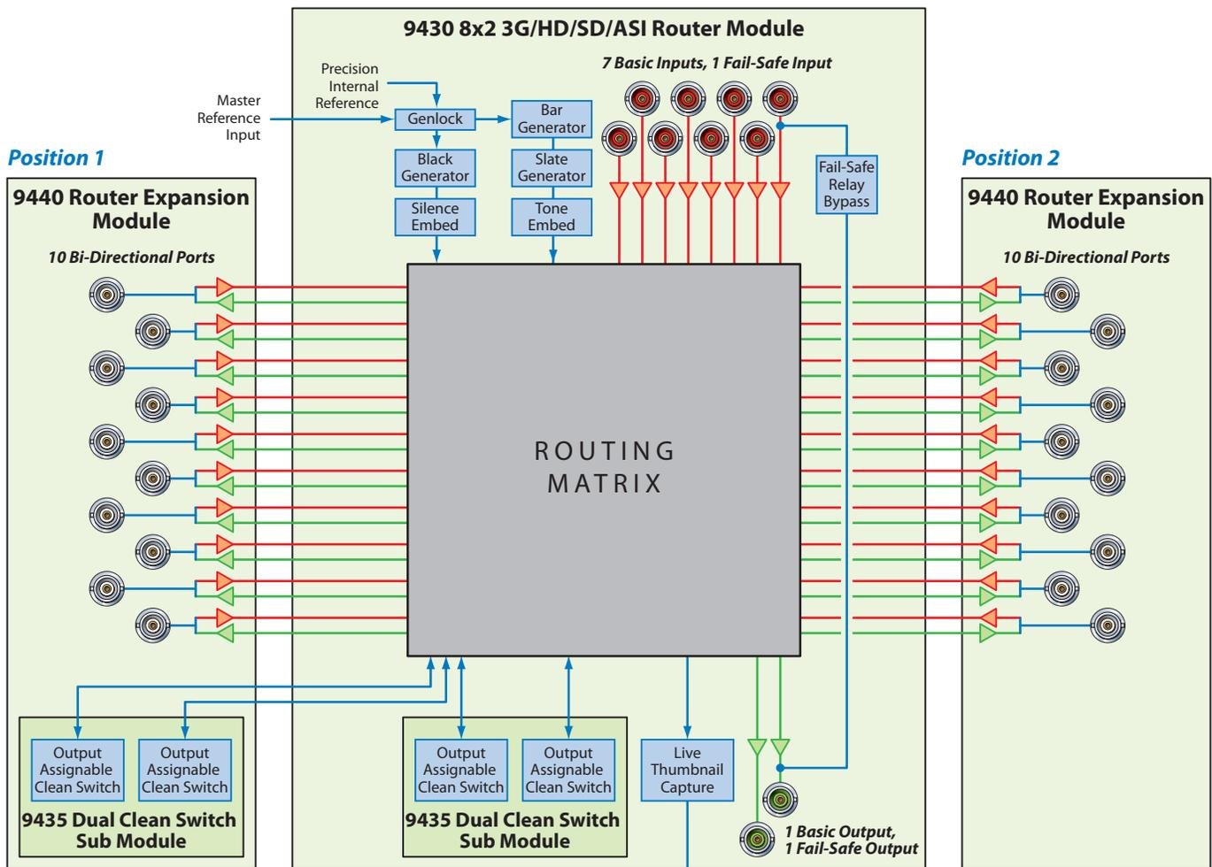
Each BNC on the 9440 Expansion Module is designated as either an input or an output. You make that assignment through the control system
