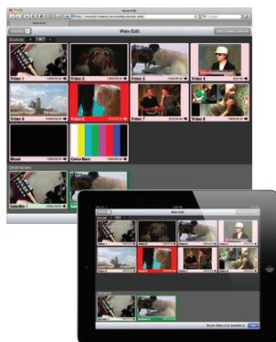
Realtime video thumbnails travel over Ethernet to the Router Control Panel where they are displayed on a compact, high resolution display. Built-in signal diagnostics show synchronicity and timing, line and frame rate, embedded audio presence or absence, closed caption information, and timecode data.
