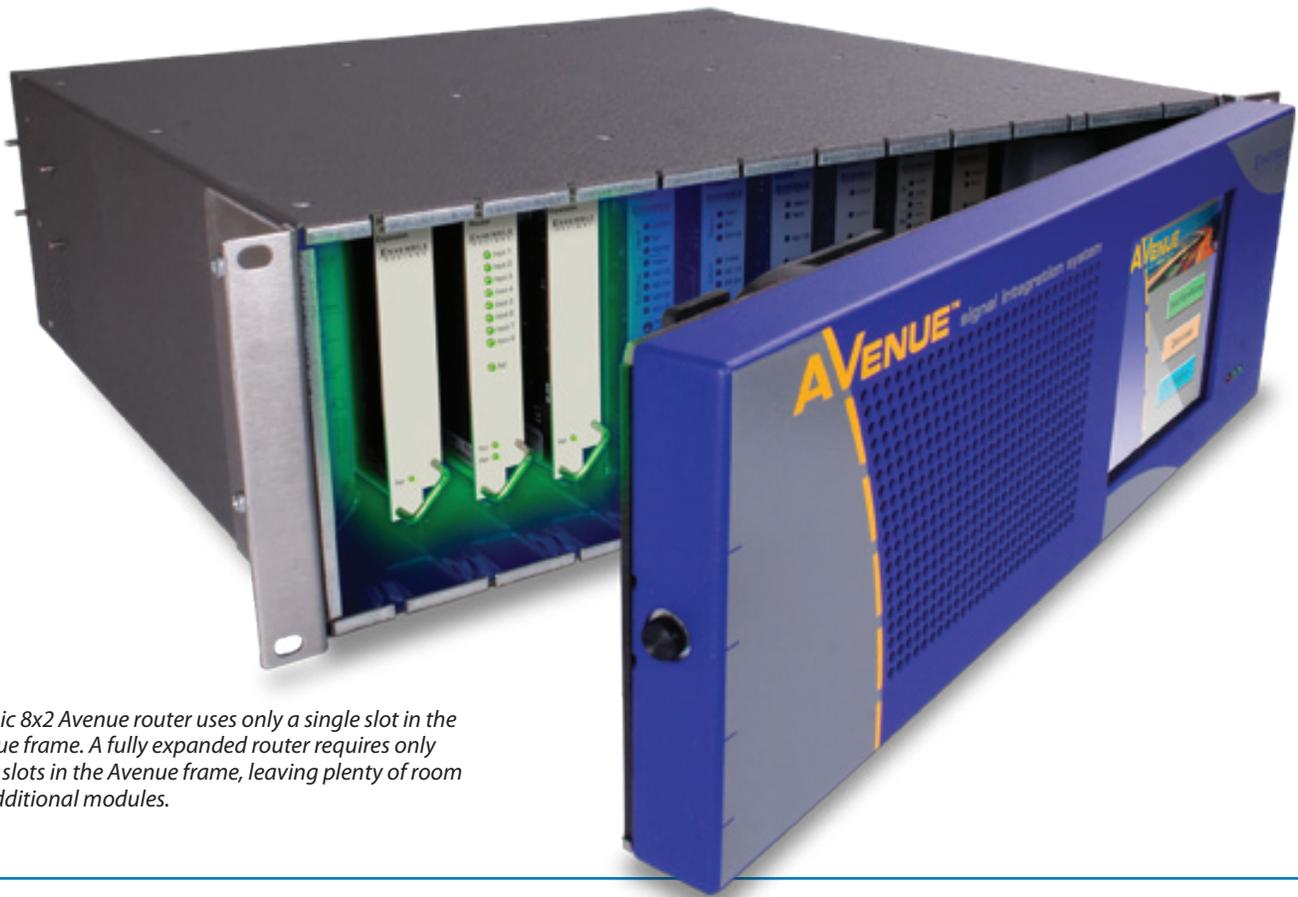
*A basic 8x2 Avenue router uses only a single slot in the Avenue frame. A fully expanded router requires only three slots in the Avenue frame, leaving plenty of room for additional modules.*
