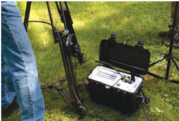
When equipped with bi-directional fiber, BrightPak supports outbound sound and picture, with return video, sound, and ifb.
